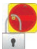
Main switch with padlock
