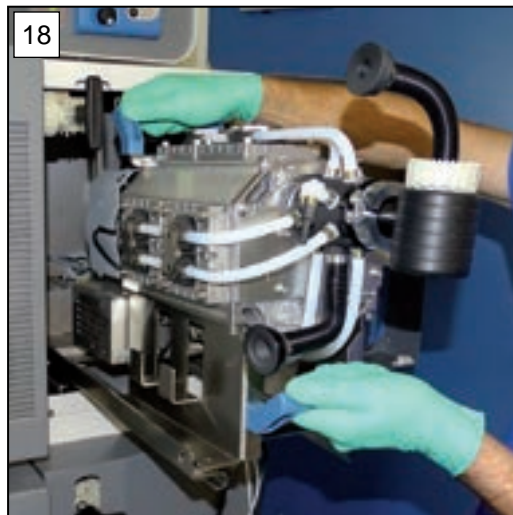
18. Take out the vacuum pump with both handles.
