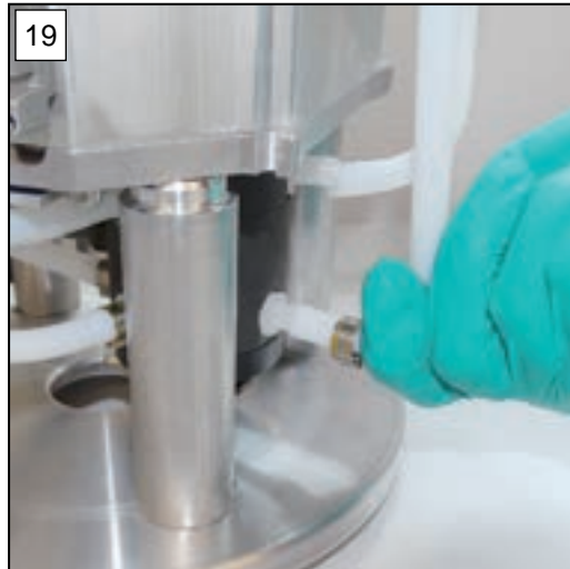
19. Slide the molded hoses back onto the hose nozzles.
