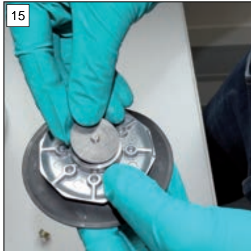
15. Place all spacer discs on the thread pin.
