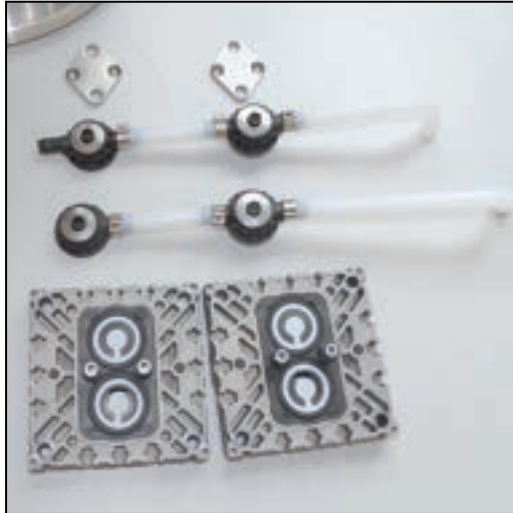
Top view: Valve terminals, valves and pump head pair.
