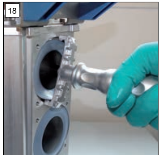
18. Initially tighten the assembly with the diaphragm wrench by hand.
