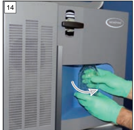
14. Screw in the condensate catch pot.
