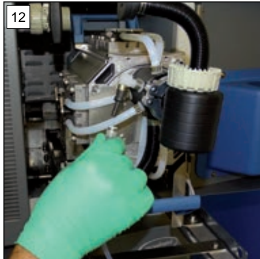
12. Push back the metal ring of the plug coupling and pull out the gas ballast hose.
