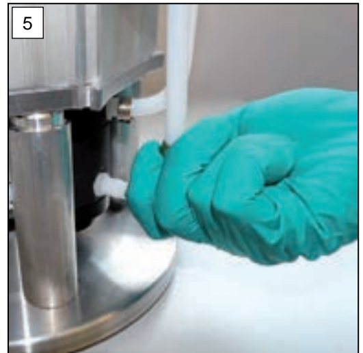
5. Pull the molded hoses off the hose nozzles.
