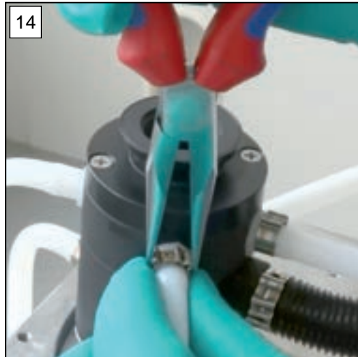
14. Slide the hose clamps onto the hose nozzle and close them with the flat nose pliers.
