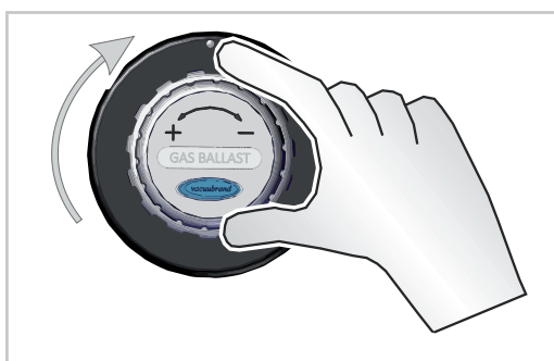
Close gas ballast valve
