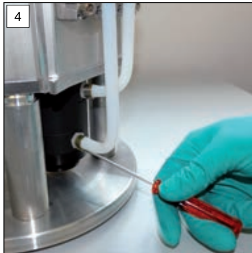
4. Open the hose clamps of the hoses of a pump head pair. Flat-head screwdriver size 1.
