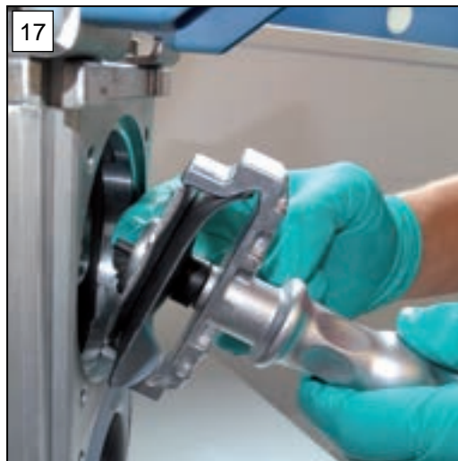
17. Hold the spacer discs firmly and place all the components carefully on the connecting rod thread.
