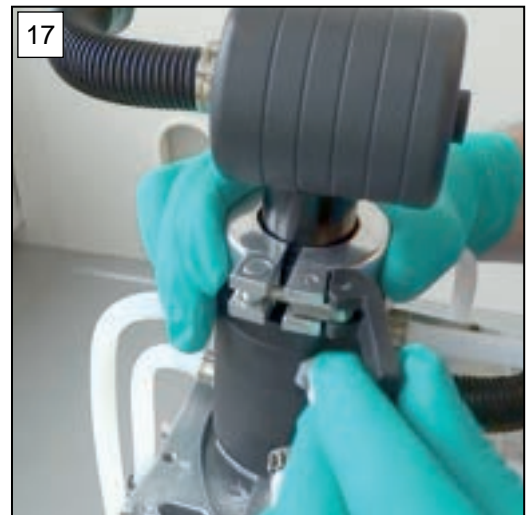
17. Place the centering ring between the flanges and fasten the outlet condenser to the suction/pressure distributor with the clamping ring.
