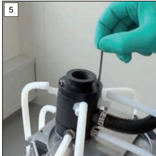
5. Pull the screws out of the pressure distributor.
