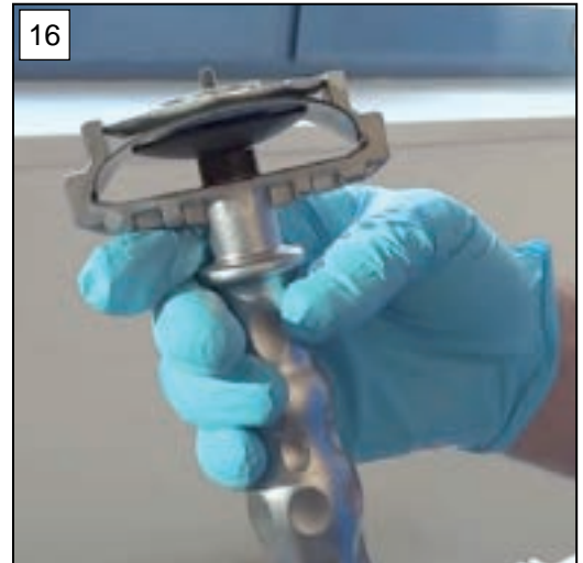
16. Secure the diaphragm assembly inside the diaphragm wrench.
