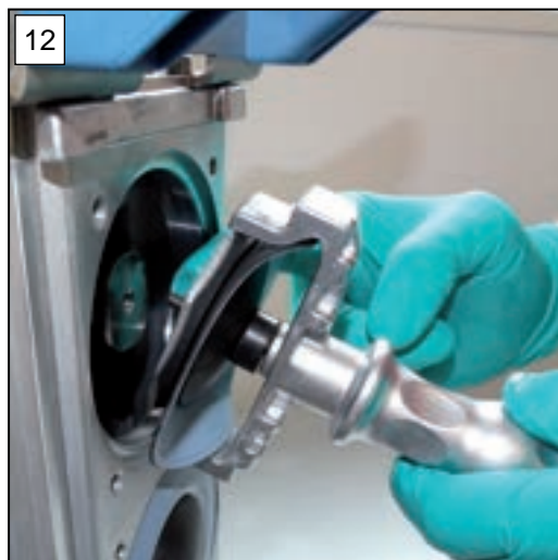
12. Lift the diaphragm along with all the parts out of the vacuum pump. If the spacer discs adhere to the connecting rod, remove them carefully.
