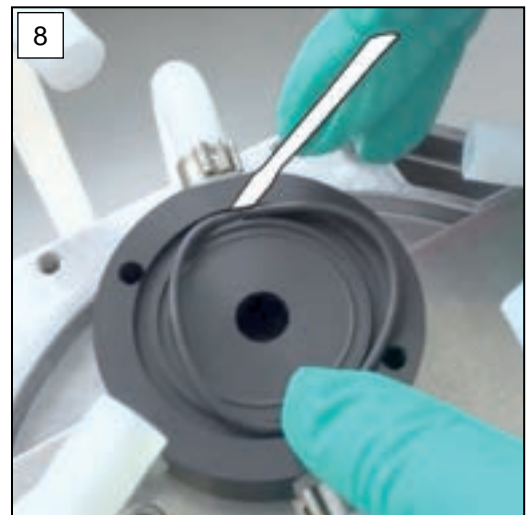
8. Carefully remove the used O-ring.
