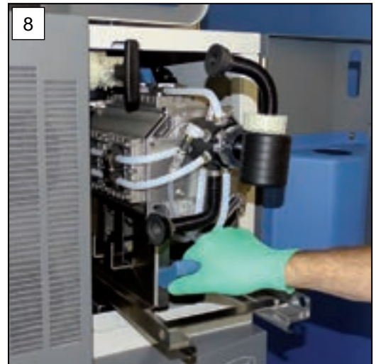
8. Slide the vacuum pump back into the pump module housing.
