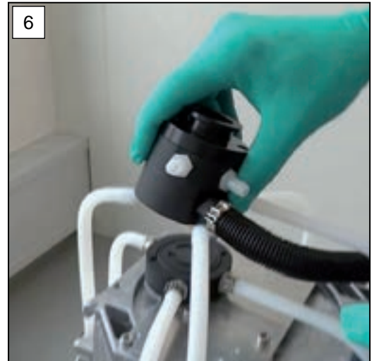
6. Remove the suction distributor and set it aside.
