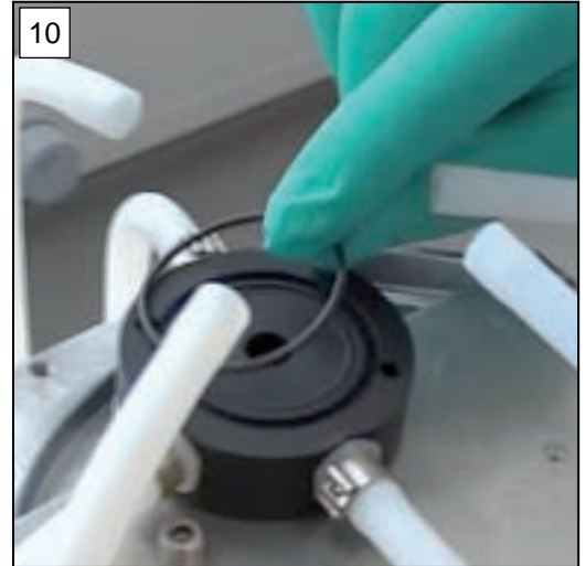
10. Place the new O-ring in the groove and press it down slightly.
