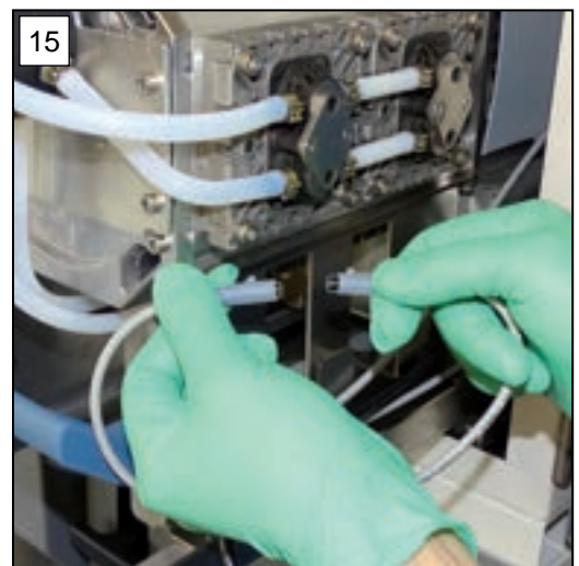
15. Disconnect the VACUU BUS cable.
