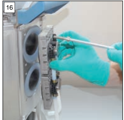
16. Hold the pump head pair at the vacuum pump and wind in the screw fittings.
