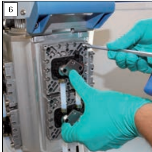
6. Unscrew the socket head screws from the head covers. Hex key size 5.
