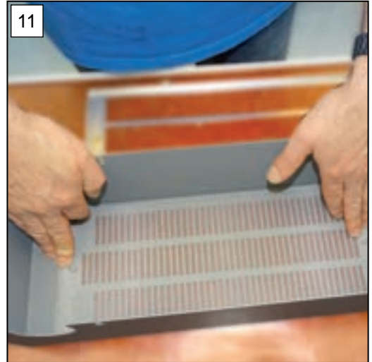
11. Place the new fan fabric in the air inlet.
