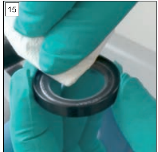
15. Clean the centering ring on both sides.
