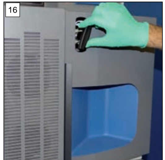
16. Turn the black handle of the isolation valve 90° in either direction.
