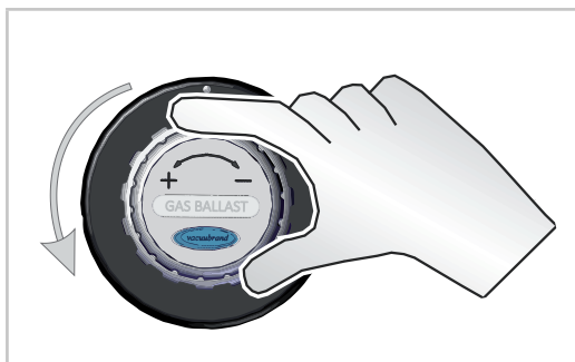
Open gas ballast valve
