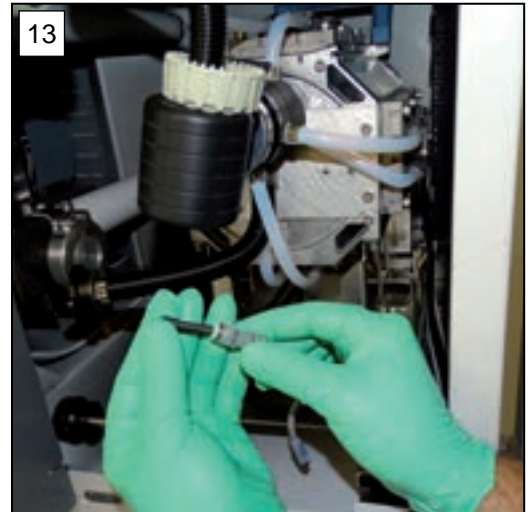
13. Close the gas ballast hose with a blanking plug.
