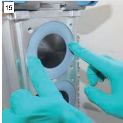
15. Carefully press the diaphragms centrally into the housing opening, ensuring they are flush with it.
