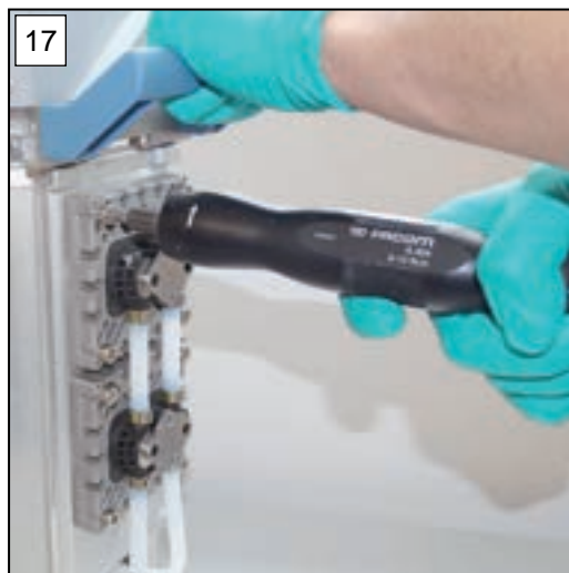
17. Tighten the screw fittings crosswise with a torque wrench of 6 Nm.
