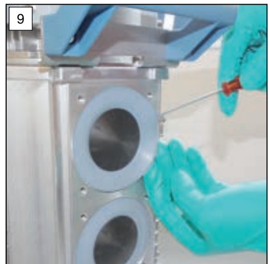
9. Carefully lift the diaphragm using an aid, e.g., a sturdy plastic rod or flat-head screwdriver.
