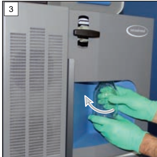
3. Screw out both condensate catch pots.
